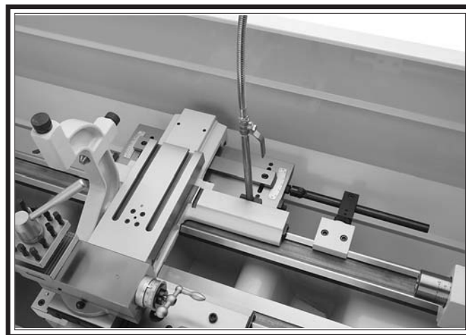
Figure 95. Model SB1271 Taper Attachment.
